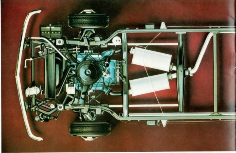
had to fulfill a variety of functions. For example, it had to be able to soak up bumpy roads, as well as cruise the Interstate. So, in the rear, you'll find four wheels in tandem. Not dual. Suspended on air, not stiff steel springs. This happy combination smooths the ride and produces a wide stance.
